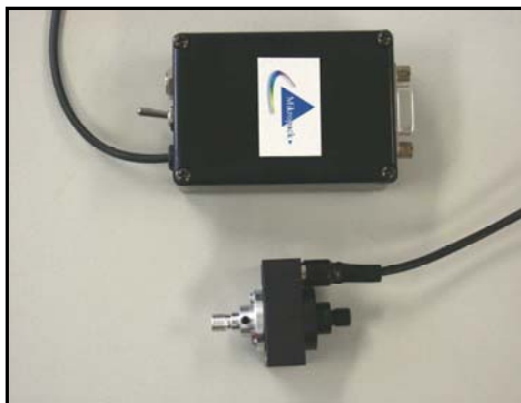
Inline TTL Shutter (bottom) with 15-pin input component and control circuitry (top)
